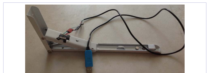
Figure 8: Experimental setup to monitor the motion of a triangular frame by GY953 module
